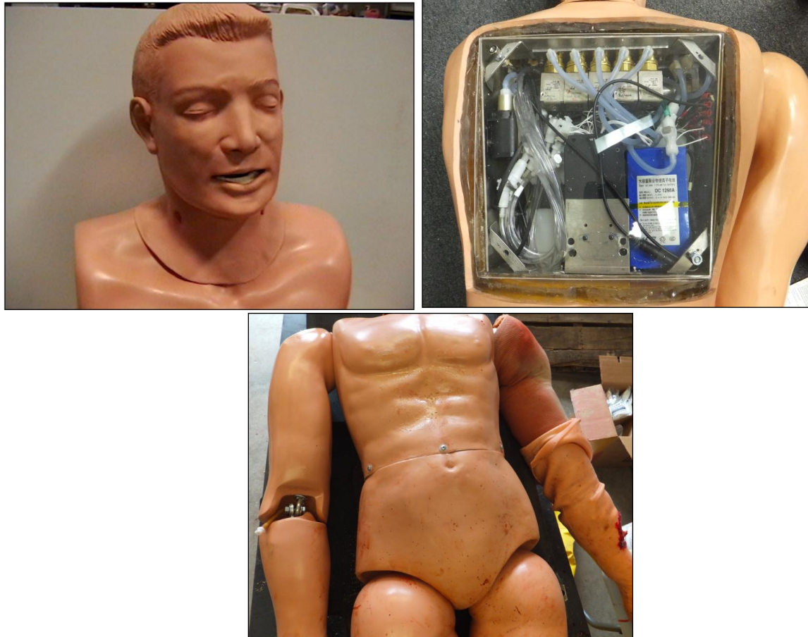
Figure 3: Rescue Randy® Modifications: New Upper Airway (Top Left), Internal Bleeding System (Top Right) and Attached Tourniquet Training Arm (Bottom)
