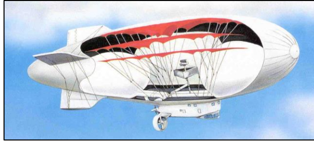
Figure 1. US Navy YEZ-2A Airship Concept in Showing Internal Structures and Surveillance Radar
