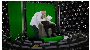
Figure 5 – Subject receiving direction in light stage used for generating 3-D imagery for holographic display
