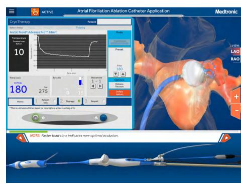
Figure 9. User Viewing Cryoballoon Temperature on CryoConsole During Post-Ablation Thaw
