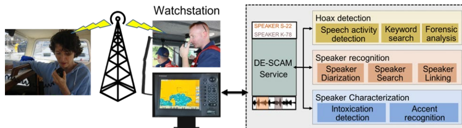
Figure 8: Conceptual diagram of the maritime VHF radio monitoring use case.
