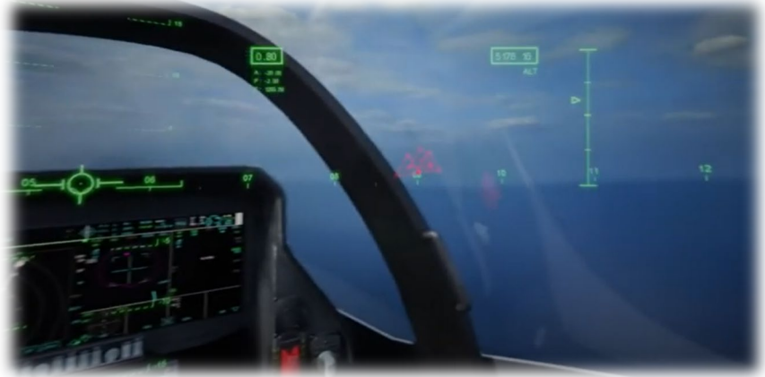
Figure 2. F-35 HMD identifying three allied aircraft noted by red triangles. Source: Collins Aerospace
