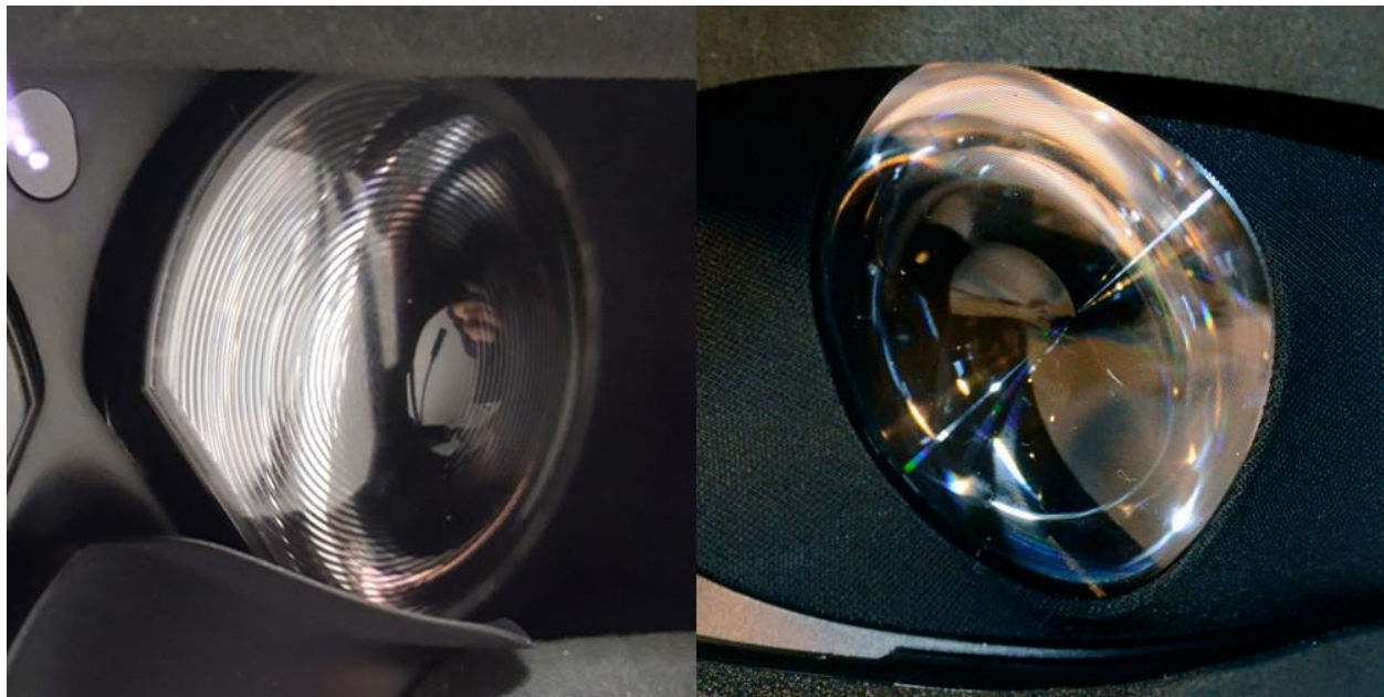
Figure 3. HTC Vive Fresnel Lens (left) and Oculus Rift Hybrid Fresnel Lens (right)
