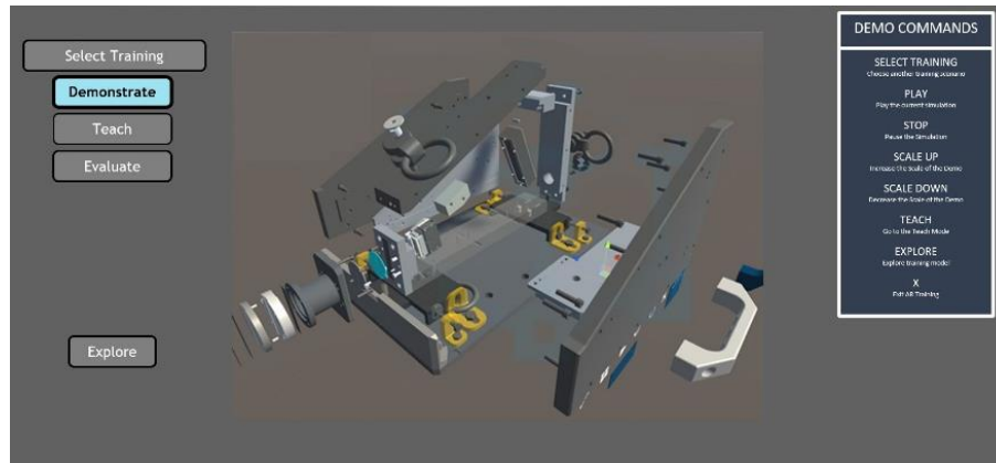
Figure 3. Learn Stage Demonstrates the Assembly and Disassembly Sequence of the 'CRITR' Assembly
