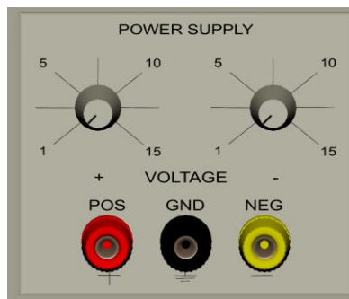
Figure 2. DC power supply section of the Digital/Analog Trainer
