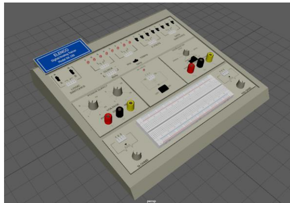
Figure 1. 3D model of the Digital/Analog Trainer in Autodesk Maya
