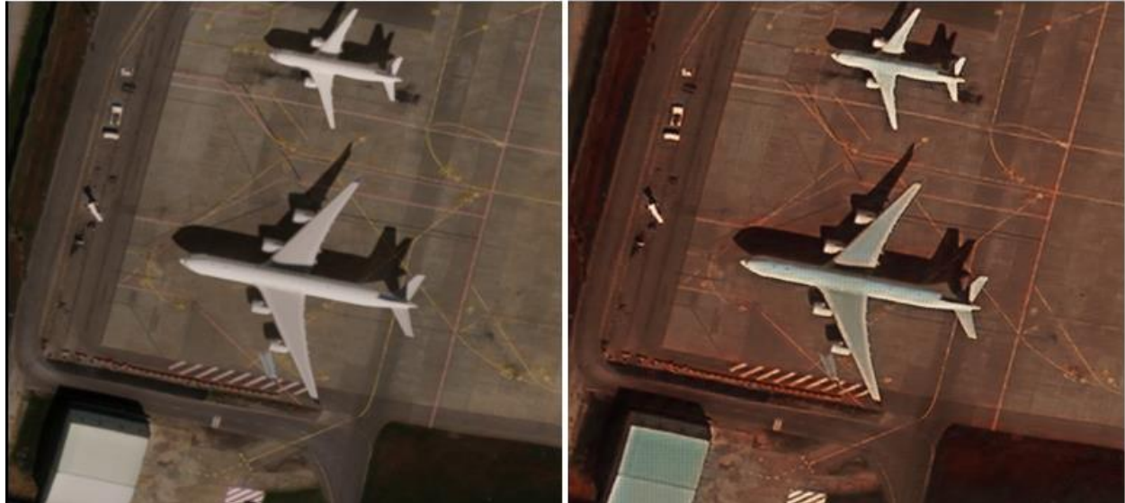
Figure 2. Left: Original Simulated Synthetic Image. Right: Resulting Image After Modifying the Original Image with GAN-based Domain Adaptation, a Post-processing Technique used to Enhance Domain Match (image from Lavander 2024).
