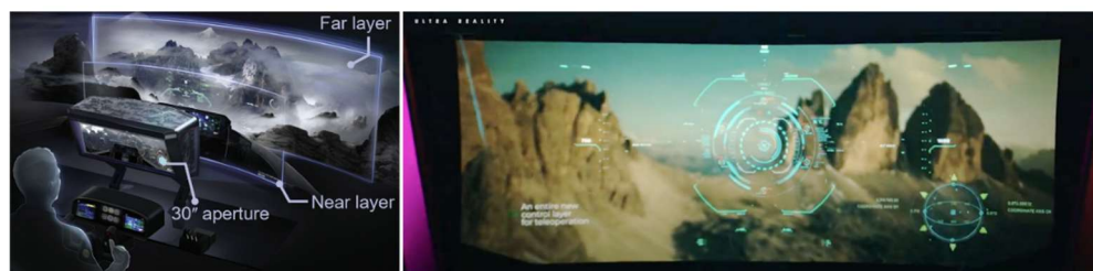
Figure 8. Dual layer extensions of UR provide multi-depth flight simulation training. Left: Concept rendering showing a synthetic environment on the far layer and HUD content on the near layer. The true-depth (monocular) image content spans a maximum of 122” and the depth ranges from 70 cm to 2.5 m. Right: Photograph of prototype, focusing on HUD content (in focus), with out-of-focus synthetic environment.
