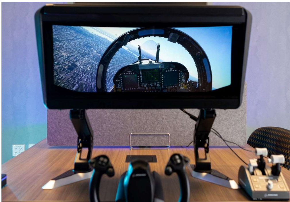
Figure 1. Brelyon Ultra Reality (UR) flight simulation platform. Note that the on-screen content is in focus, whereas the hardware itself (the surrounding housing, for example) is slightly blurred. This demonstrates that the image is optically deeper than the aperture, as the camera focused farther to capture it clearly.
