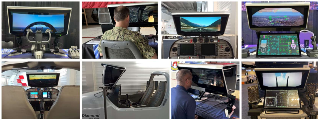
Figure 6. User evaluations testing of Ultra Reality flight simulator including COTS instrumentation and integration into larger flight simulator hardware. Systems integrations include COTS instrumentation (instrumentation cluster, yoke/throttle, etc.), FFSS, and pre-existing synthetic content.
