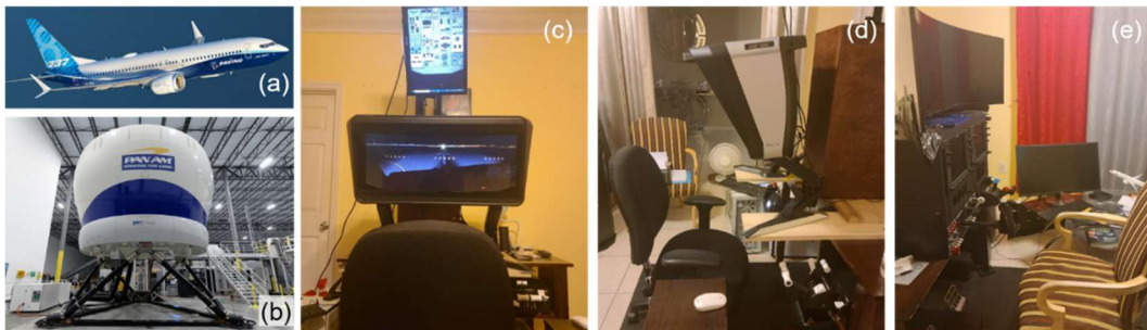
Figure 7. Comparison of different flight training methods to UR. (a) Physical 737 Max, (b) FFS. (c), (d) UR platform. (e) Samsung 55" curved monitor.
