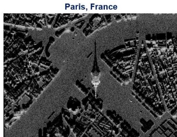
Figure 2: Simulated SAR Image Demonstrating the SAR Overlay Effect (RFView)
